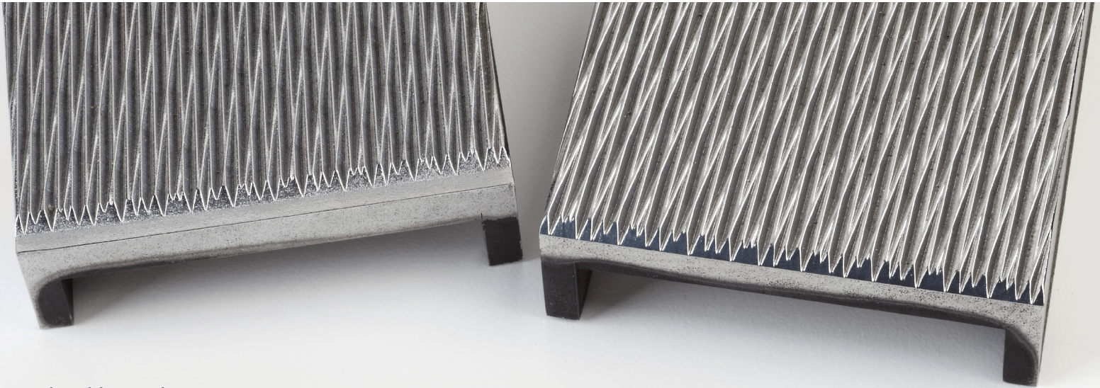
Industrial die, printed using LPBF
