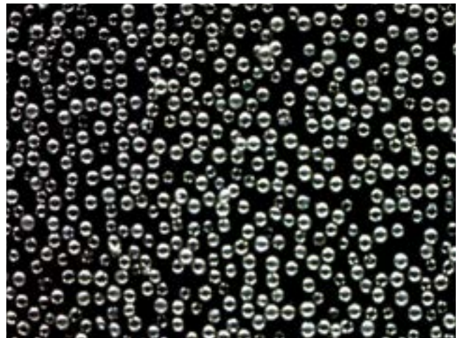
Optical image shows the spherical morphology of EverShot™ 20A
