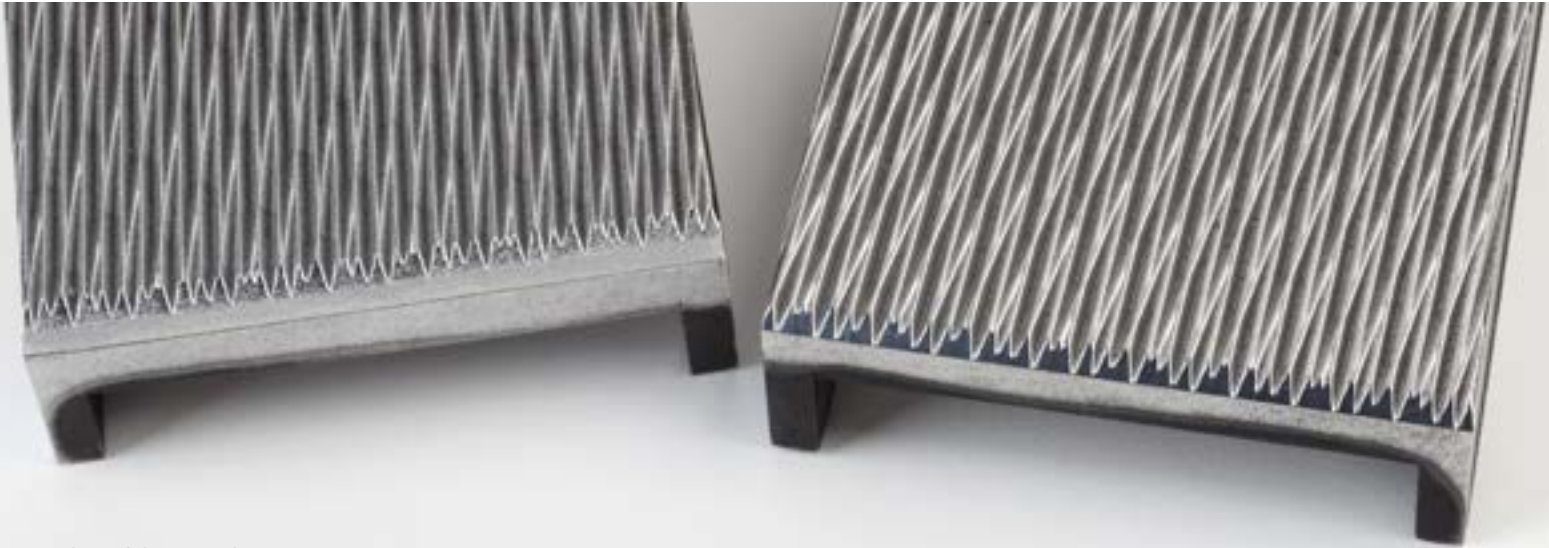
Industrial die, printed using LPBF
